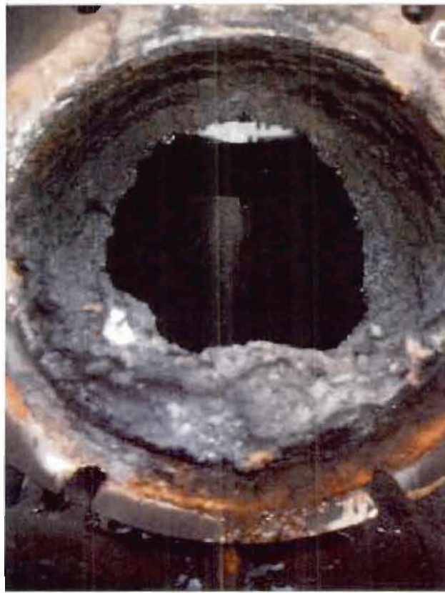
Fig. 14 Gooseneck Fitted with SelfClean Sprays after 30 Days Without Any Cleaning
